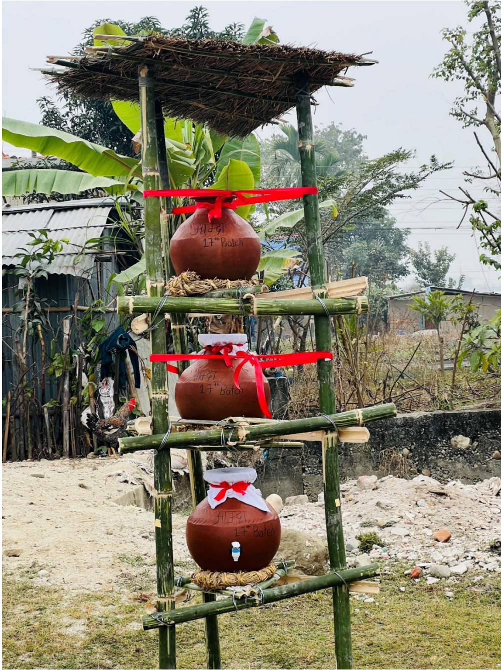
Image 3: community Health Action Group A ( Water Purification by Charcoal Filter )
